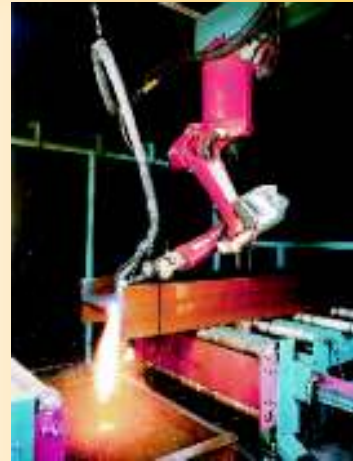
Plasma cutting with robot
